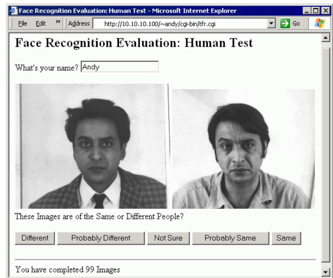
Fig. 1. Screenshot of the software application for the testing of HFR performance. After logging into the application, participants were presented a series of pairs of images and were required to choose one of the selections. Instructions were to strive for “accuracy,” and no time limit was given.
